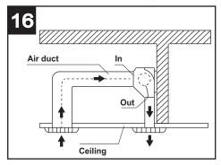
**NOTE:** if mounting above the ceiling, appliance performance could vary with respect to the stated values.
